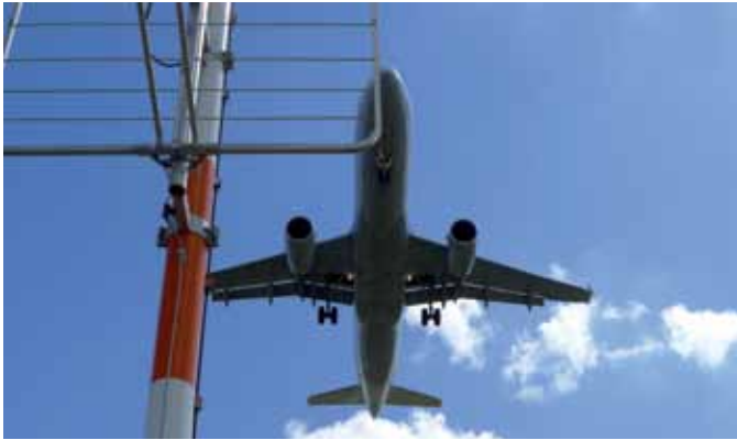
An aircraft lands over an antenna used for monitoring the correct functioning of the localizer
